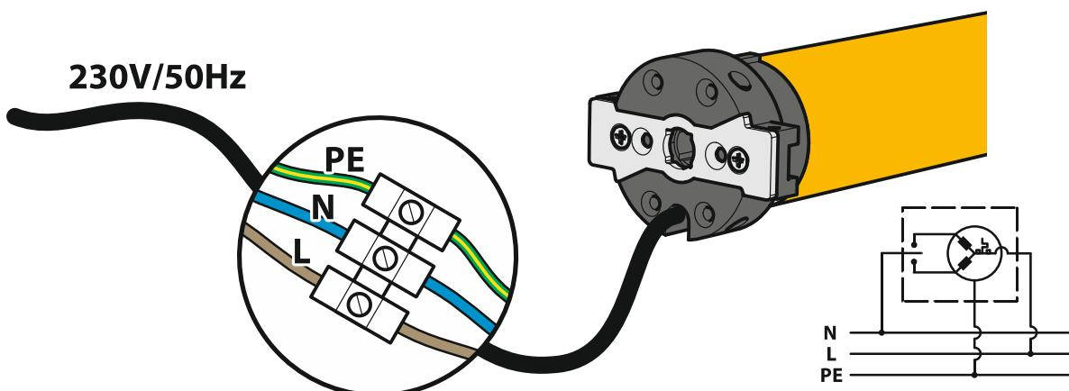
**Fig.1 – Electrical interfaces**
