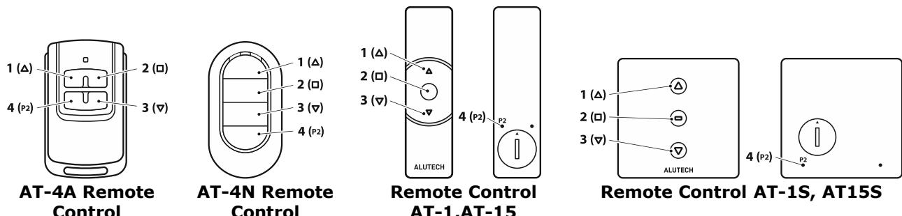
**Fig.2 – The appearance of remote controls and key assignment:**
