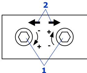
**Fig.3 – Limit switch adjustment**
